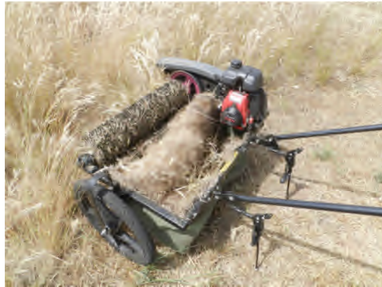
Figure 14: Hand-propelled 'Grass Grabber' Figure 15: Grass Grabber, cover off, seed tray full
