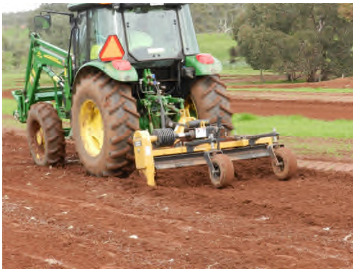
Figure 31: Preparing the seed bed with a power rake and tractor (Mine Rd SEB-Offset areas)
