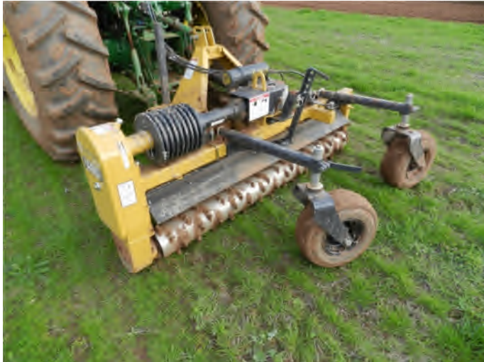
Figure 32: Power rake and tractor used to finely cultivate the seed bed to a depth of 25-30mm
